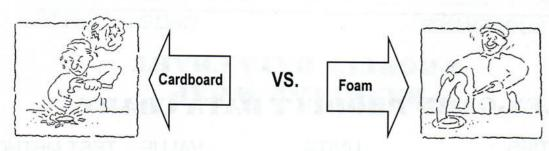
FLEX-GARD is made of foam. It will not stick to cement like cardboard. Spacer removal is fast and easy. Plus, FLEX-GARD cost no more than conventional cardboard spacers.
